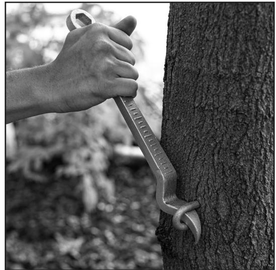
**Step #2** With your pilot hole already drilled per the hardware manufacturer's specification, begin turning the lag screw into the tree by hand until you can no longer easily rotate it.
