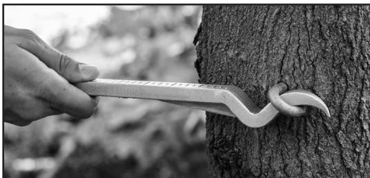
**PLP Tip:** Install the TREE-GRIP™ Dead-end, thimble, and cable. Reference the TREE-GRIP Dead-end application procedure (SP2056).
