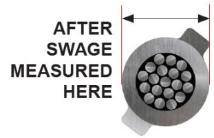
Figure D. Measure the fitting as shown after the first swage. Adjust the tool accordingly before completing any additional swaging.
