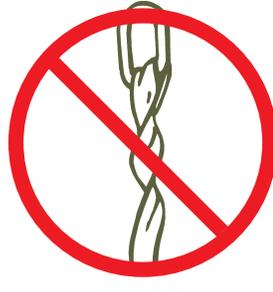
*A sling shall not be pulled from under a load when the load is resting on the sling.*
