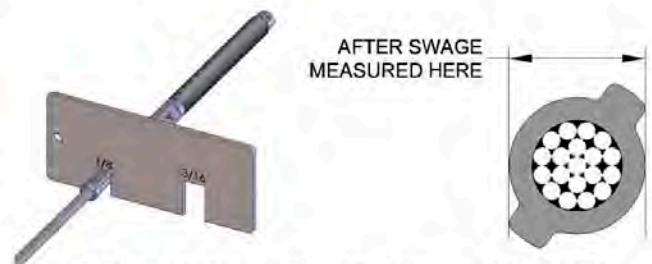
Figure D. Measure the fitting as shown after first swage. Adjust the tool accordingly before completing any additional swaging
